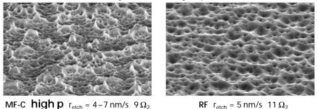
MF-C high p  $r_{etch} = 4-7 \text{ nm/s} 9 \Omega_2$
